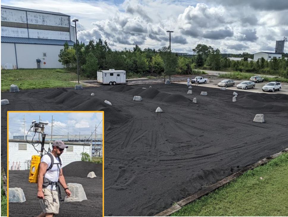
Mike tests the KNaCK (Kinetic Navigation and Cartography Knapsack)
